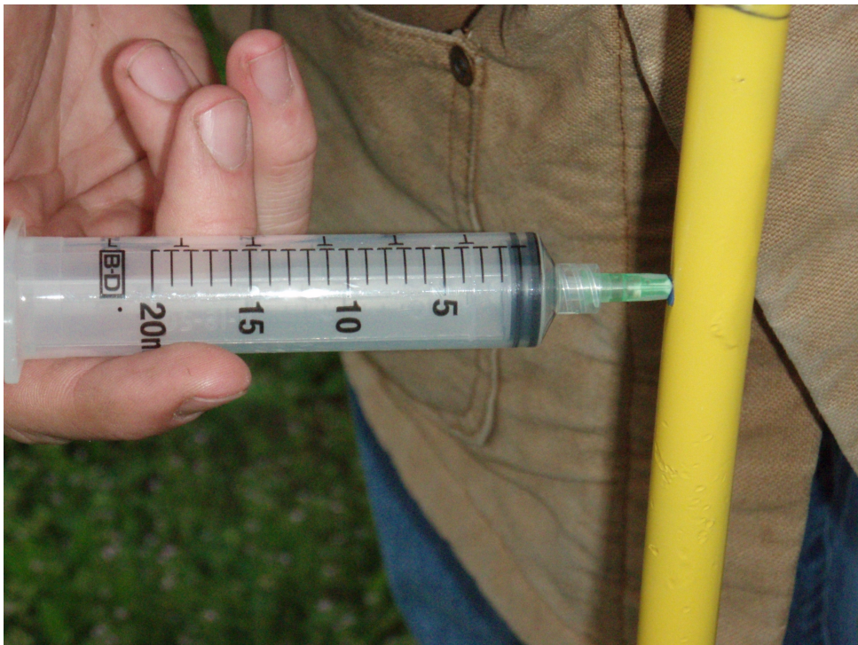
Figure 8: Atmospheric pressure forcing plunger to bottom syringe signifies no leaks
