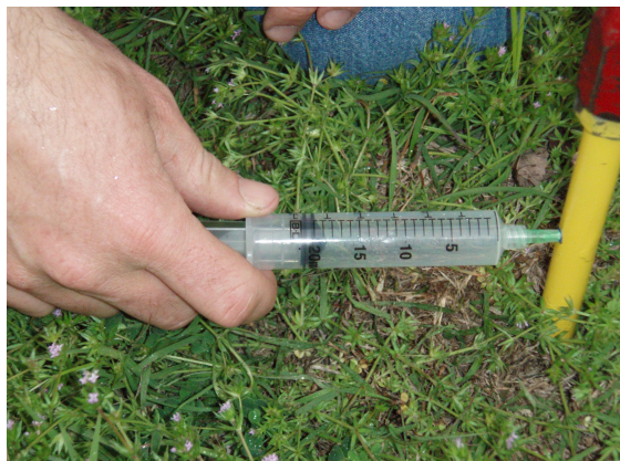
Figure 10: Probe at 1m and full sample syringe
