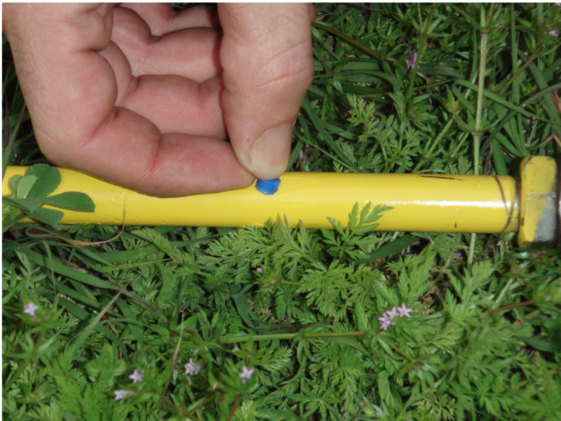
Figure 2. Push Septum into hole
