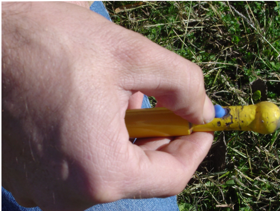
Figure 6: Sealing Probe Inlet
