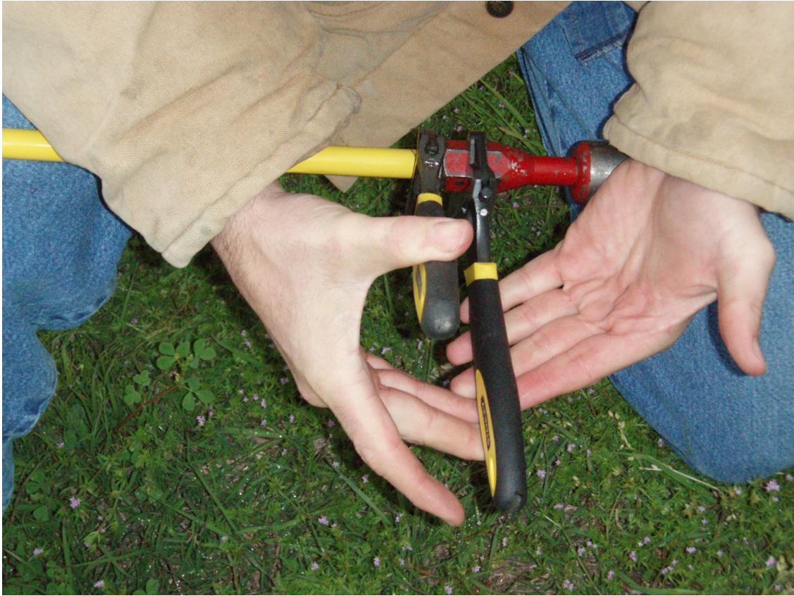
Figure 1. Tighten lock nut
