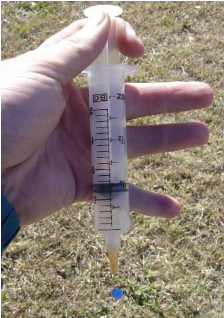
Figure 9: Leak test syringe
