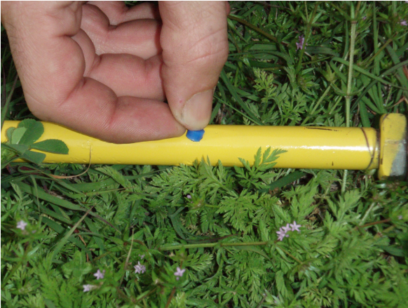
Figure 4: Pushing Septum into probe
