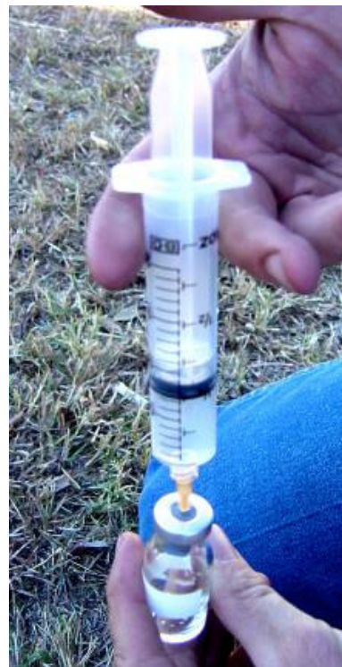
Figure 11: Inject all of sample in bottle
